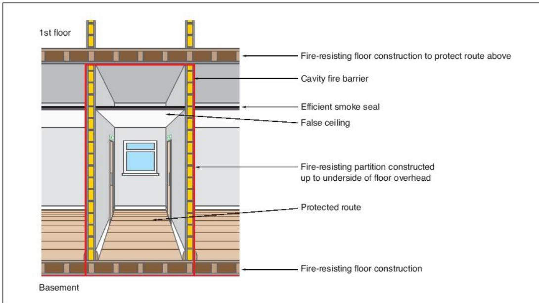
Figure 1: Fire-resisting construction
