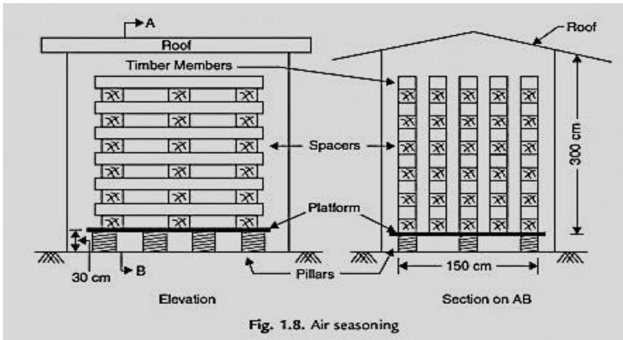
(iii) **Artificial Seasoning:** In this method timber is seasoned in a chamber with regulated heat, controlled humidity and proper air circulation. Seasoning can be completed in 4 to 5 days only. The different methods of seasoning are:
