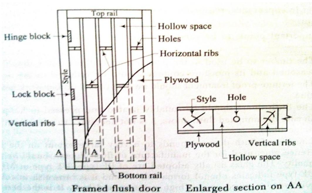
It consists of styles, rails, horizontal ribs, vertical ribs, and plywood. As shown in fig.
