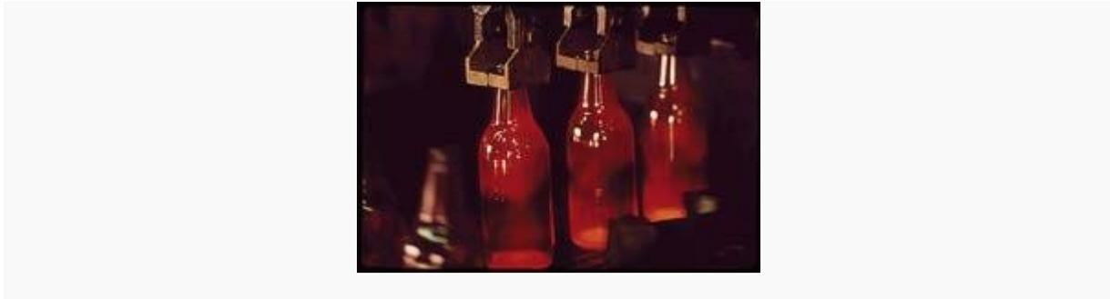
There are, currently, two primary methods of making a glass container: the blow and blow method, used for narrow-neck containers only, and the press and blow method used for jars and tapered narrow-neck containers.
